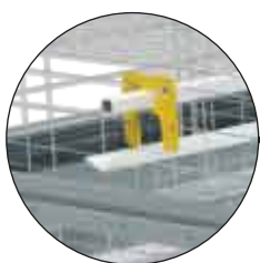
Drinking line on each floor
